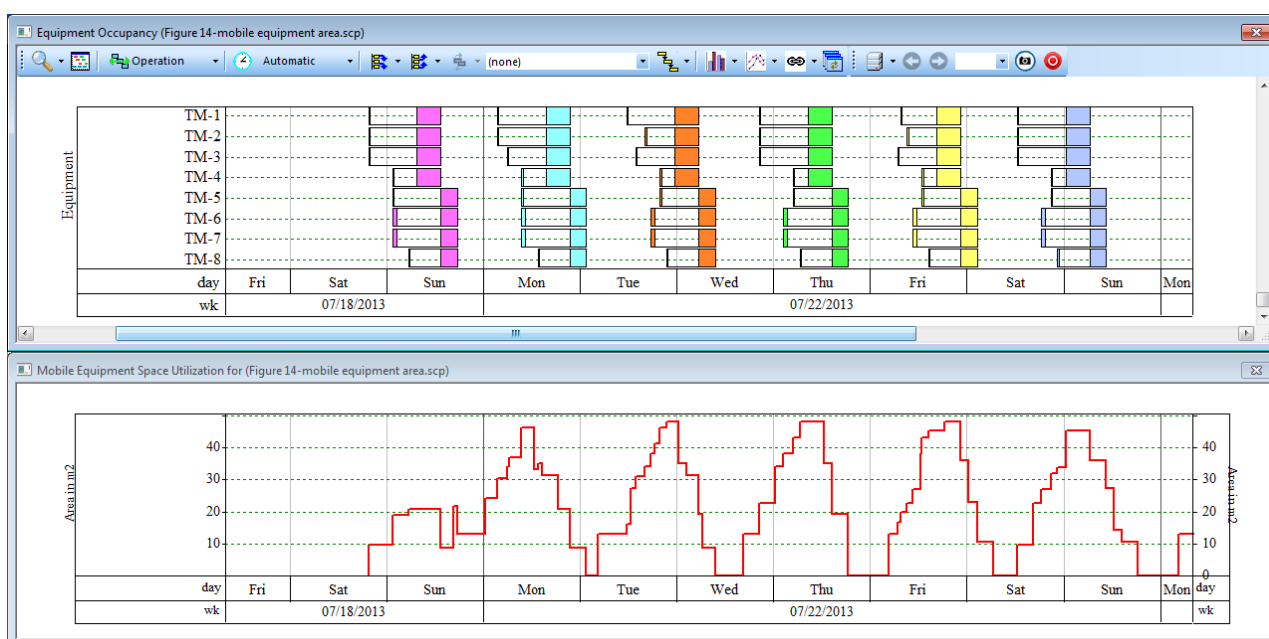
Figure 15. Mobile equipment floor space requirement.
