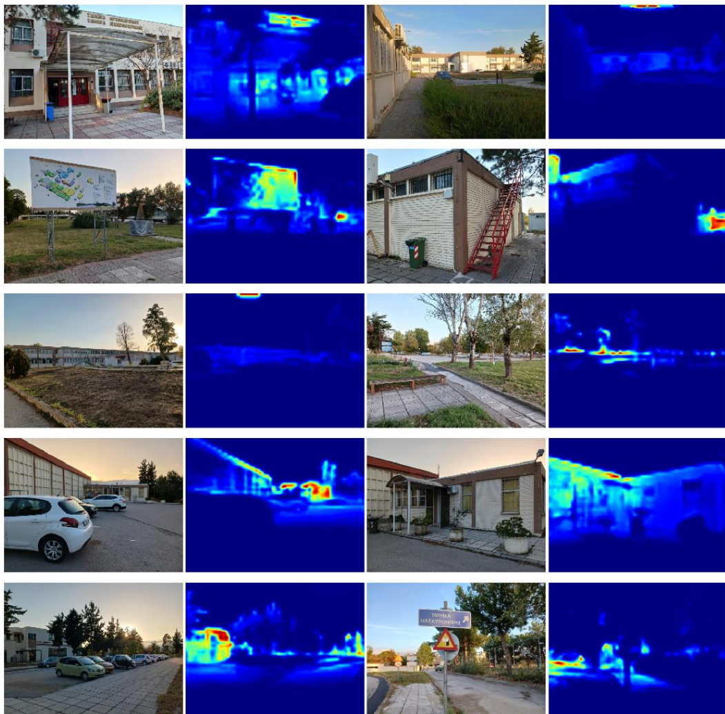
Figure 5.16: Prediction on IHU with LapDepth (Columns 1 and 3: RGB images. Columns 2 and 4: predictions)
