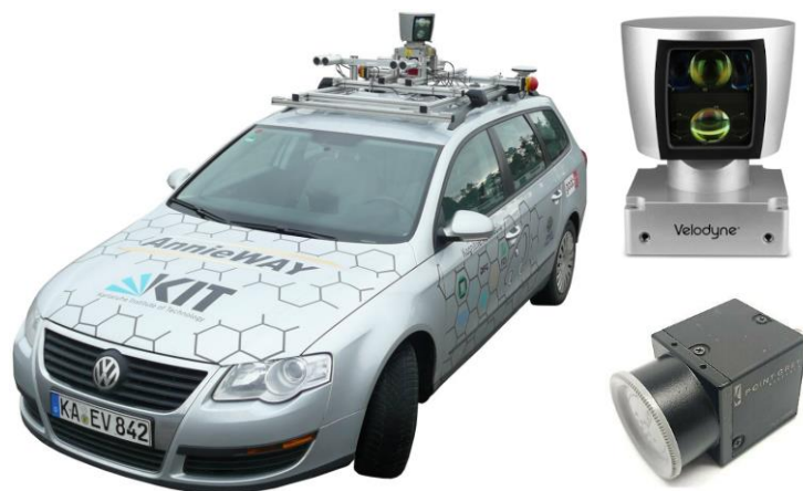
Figure 5.3: KITTI recording equipment [60] [61] [62]
