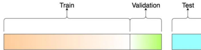
Figure 3.11: Training, validation, test set splits [44]
