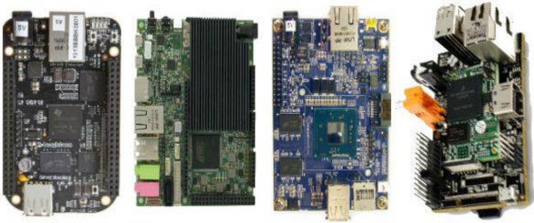
Figure 34: BeagleBone Black, UDOO, MinnowBoard Max and HummingBoard (left to right)
