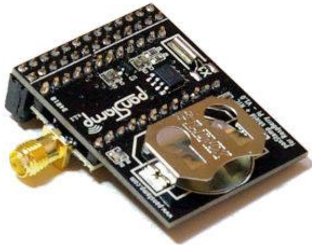
Figure 26: PanStamp shield for the Raspberry Pi [35]
