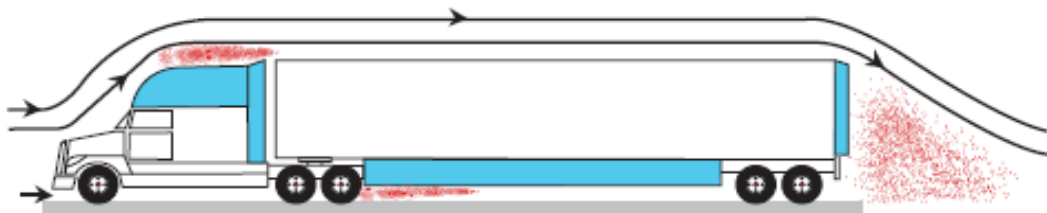
B: A tractor-trailer with aerodynamic devices installed produces less drag (shown as shaded area)
